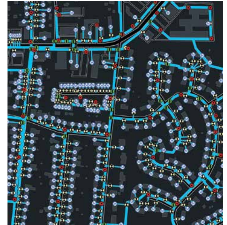
Above: The ArcGIS Utility Network offers comprehensive visualisation and analysis of the network system. For example, dynamic tracing enables water utilities to determine the exact valves to shut off when a pipe bursts.
